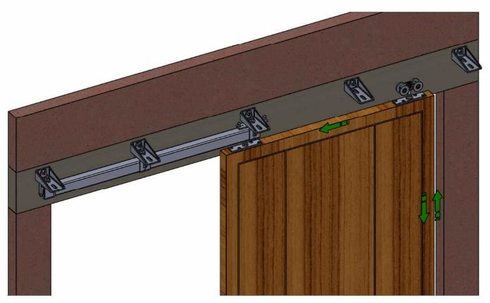
Insert the first track through the brackets making sure it fits into the closed end piece. You might have to disassemble some of the brackets for easy access as shown in fig.14.
