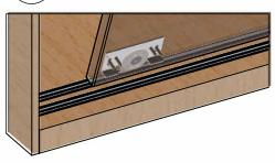
$\begin{pmatrix} 6 \end{pmatrix}$  Insert the door and slide the guides into profile. Tighten the screws (4x15mm, wood screws)
