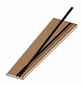
Prepare the door, position the rollers and fix them with screws ( $\phi$  4x15mm)
