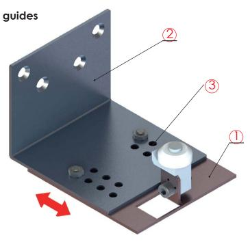
It is possible to use doors between the thickness of 20 and 50 mm. To adjust the upper rollers let the parts 1 and 2 slide to have the holes of the part 1 corresponding to the holes (3) of the part 2 referred to the correct thickness.
