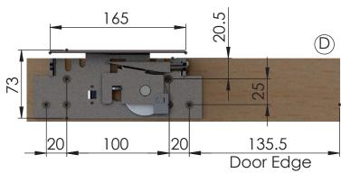
On the bottom of the outer door and fix the lower guides
