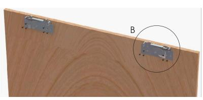
Go on top of the inner door and fix the left and right rollers
