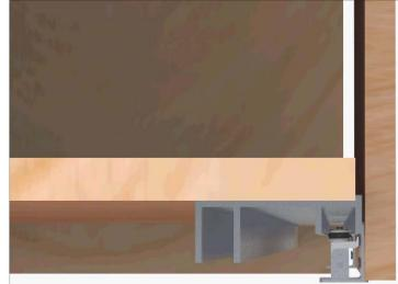
Once the top rollers are in position on the top track, push the lower guides in the bottom track outer channel untill you hear a 'CLICK' sound
