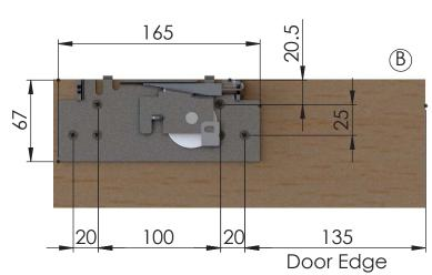
Go to the bottom of the inner door and fix the left and right lower guides
