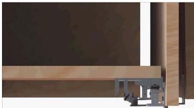
Once the top rollers are in position on the top track, push the lower guides in the bottom track inner channel untill you hear a 'CLICK' sound
