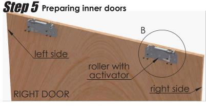
Go on top of the inner door and fix the left and right rollers.
