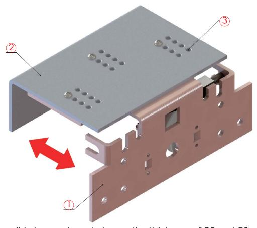
It is possible to use doors between the thickness of 20 and 50 mm. To adjust the upper rollers let the parts 1 and 2 slide to have the holes of the part 1 corresponding to the holes (3) of the part 2 referred to the correct thickness.
