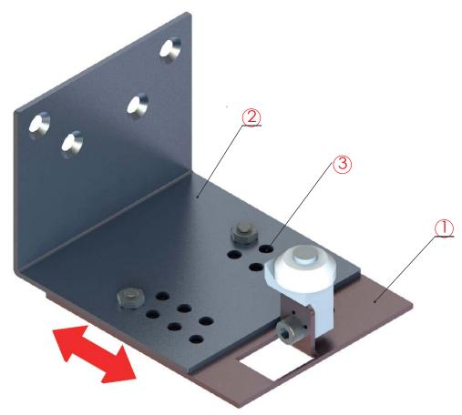
To adjust the lower guides of the outer door, let the parts 1 and 2 slide to have the holes of the part 1 corresponding to the holes (3) of the part 2 referred to the correct thickness.
