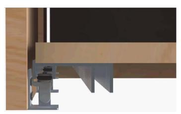
Once the top rollers are in position on the top track, push the lower guides in the bottom track outer channel untill you hear a 'CLICK' sound
