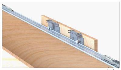
**Step 7** Mounting the left inner door - Bottom
