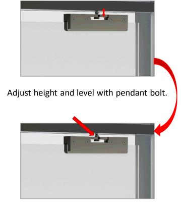
Secure position by tightening nut.
