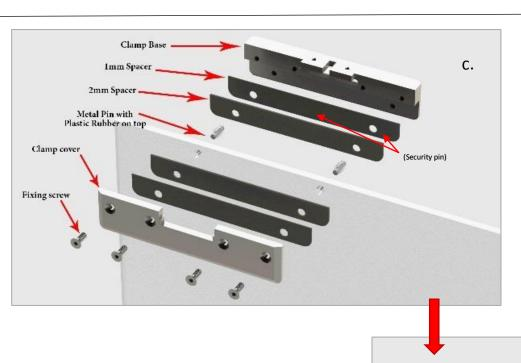
DT=8mm = > 2x 2mm spacer DT = 10mm => 1x 1mm spacer + 1x 2mm spacer DT=12mm => 2x 1mm spacer
