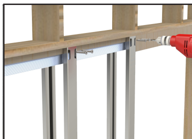
Stud frames, floor plates and door guides
