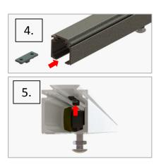
Make sure soft closer trigger is in open position then insert soft closer inside track (3.), next insert actuator in track(4) (see position on next page) and secure with screws.
