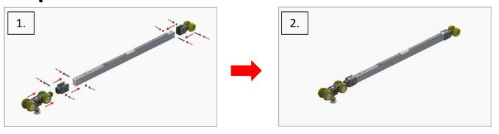
Attach 2-wheeler to the back of the soft closer. Attach adaptor to other side of soft closer, afterwards attach hanger to adaptor (1.).
