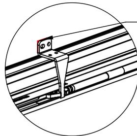
Mark the activator for fixing point, Ensure the door closed fully in a desired state.
