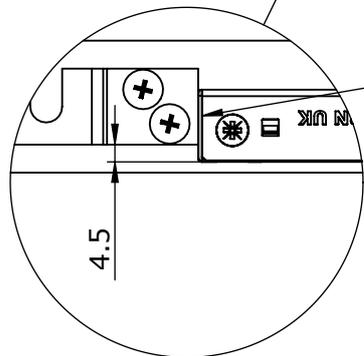
Soft closer mechanism to be butted up to door plate piece in door closing direction as shown in the figure.
