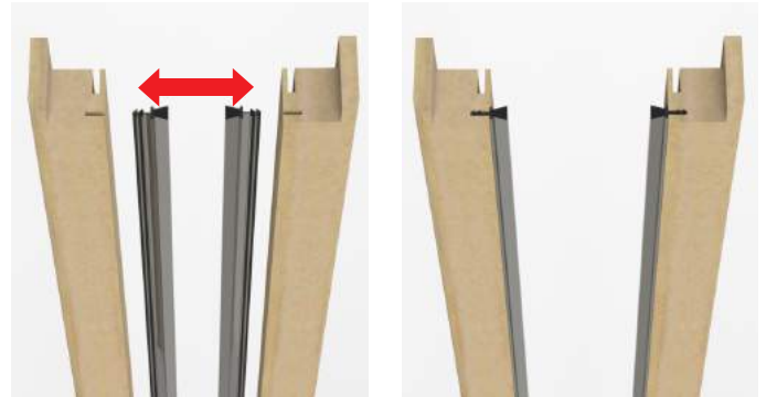
Brush seals (4) into Intermediate stud jambs (3).
