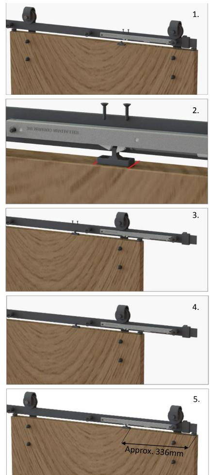
2. With the door in fully closed position and the soft closer in a closed position (spring and piston are not in tension) place actuator on top of door and in the soft closer trigger. Mark the position. It should be approx. 336mm
