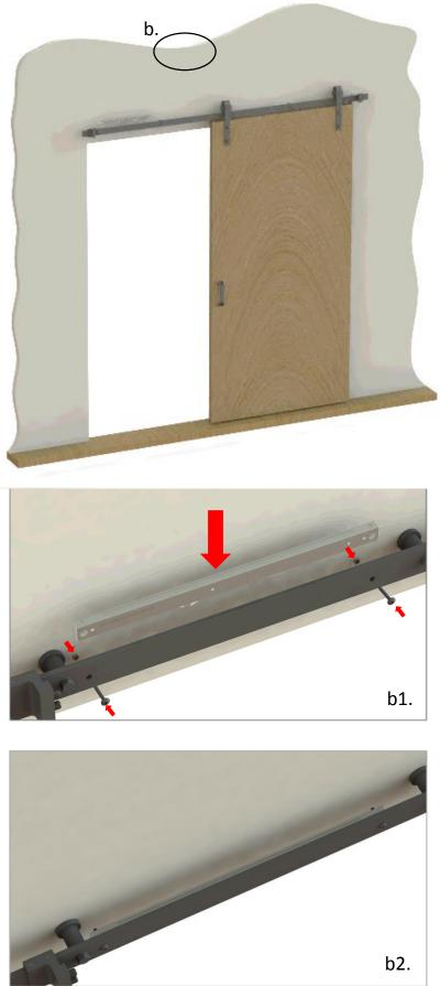
Place soft closer behind track and secure with nuts and screws. After securing soft closer make sure door is in fully closed position
