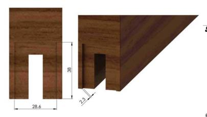
Mortice 2.3mm in depth, 28.6mm wide and 38mm high
