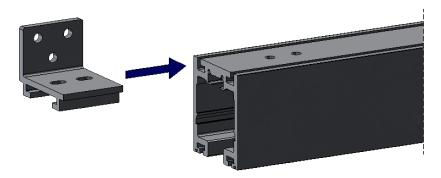
Step 2: Slide Brackets into the aluminium track
