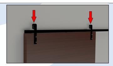
Position the hangers over track and without damaging the track slowly lower the door and hangers onto the track until they sit on the top of the track
