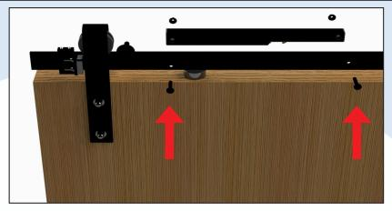
Position the soft closer on to the back of the track, with the trigger facing the top of the door. Fix and secure the soft closer with the nuts and screws provided using the holes drilled eariler.
