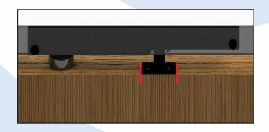
Mark out the actuator position on the top of the door.
