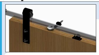
Move the door away from the soft closer. Put the packer underneath the actuator and secure the actuator in postion with the screws provided.
