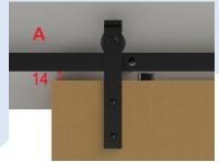
Note: Distance between the top of the door and the bottom of the track should be 14mm.
