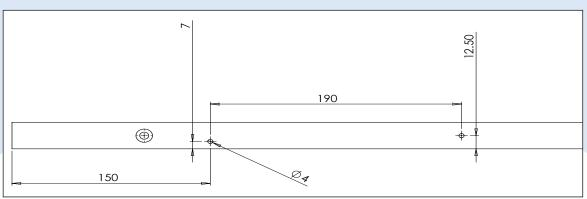
Drill 2x 4mm holes. First hole 150mm from the end of the track and 7mm above the bottom of the track. Second hole 190mm across from the first hole and 12.5mm above the bottom of the track.
