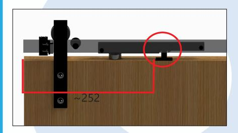
Slide the door to the end of the track. With the soft closer in the closed postion (trigger in the released state as illustrated).
