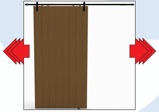
Slide the door to the closed postion and check that the actuator and soft closer are working together.
