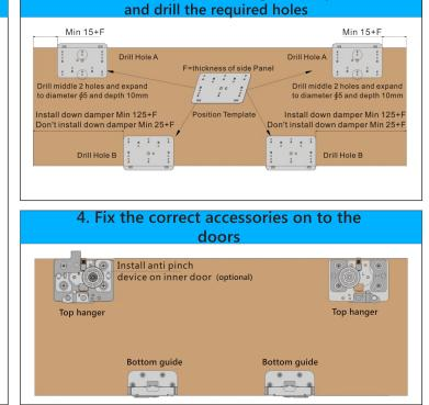
3. Locate hole position using the template
