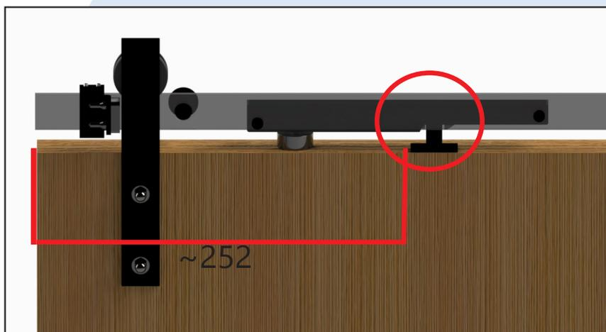
Slide the door to the end of the track. With the soft closer in the closed position (trigger in the released state as illustrated).
