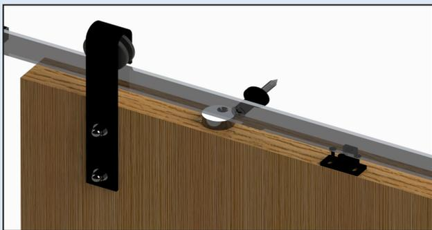
Move the door away from the soft closer. Put the packer underneath the actuator and secure the actuator in position with the screws provided.
