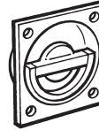
ALUMINIUM, CAST, 65 x 65mm. WHEN USED WITH 95-658 MORTICE LATCH MINIMUM DOOR THICKNESS 38mm S.A.A. 95-631 FLUSH RING HANDLE
