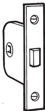
BRASS BOLT AND FOREND. FLAT FOREND, 140 x 30mm STEEL CASE. DEPTH 64mm HEIGHT 70mm THICKNESS 14mm BACKSET 43mm 95-657 MORTICE LATCH
