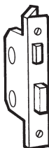
BRASS BOLT AND FOREND 3 LEVERS. HALF REBATED FOREND, 120 x 30 x 13mm. STEEL CASE. DEPTH 50mm. HEIGHT 70mm. THICKNESS 14mm BACKSET 57mm. KEYHOLE/FOLLOWER CENTRES 57mm 95-647 REBATED MORTICE LOCK
